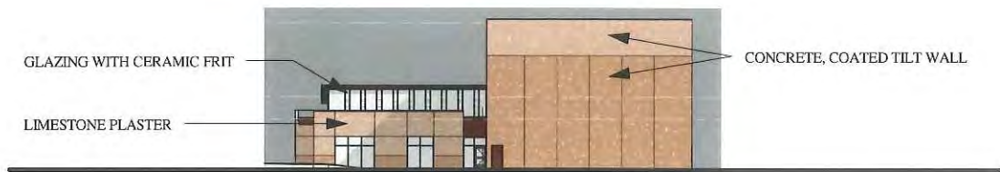
West Building Elevation
